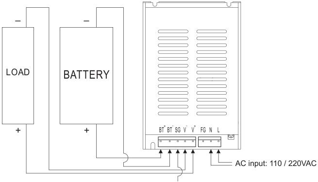
Power source normal: SG contact is open circuit to ground. Green LED on, Red LED off. Power source failure (battery powered): SG contact is short circuit to ground. Green LED on, Red LED on.
